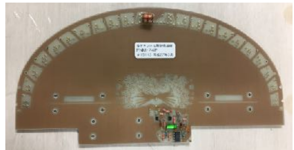
Prototype of field mapping probe
