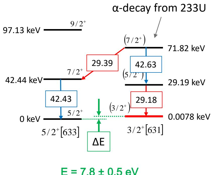
Detection of Internal conversion electrons from isomer state
